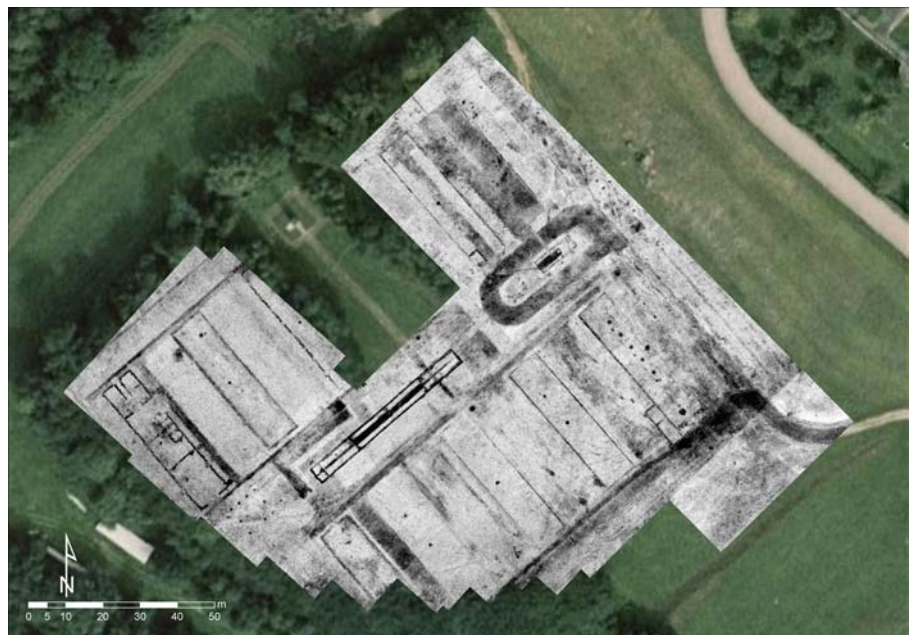
Fig. 8. Georadar map from the hospital camp at Mauthausen with the foundations of the barracks (by Archaeo Prospections®).
