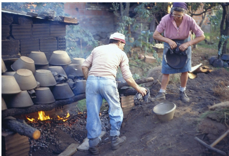
Molelos black pottery firing process (© C.M. Tondela).
